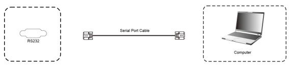
After using serial port cable to connect central control equipment and machine, certain function of the machine can be controlled via central control equipment, such as: machine ON/OFF, and adjustment of sound volume, etc.
